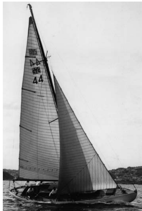
Yacht Rani , rigged as a cutter, showing two head sails in left photo, and in the right photo showing only one head sail, and consequently could be said to be sloop rigged.
