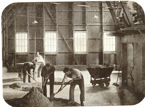
One of the Sampling Floors, showing Cornish Quartering Method of taking samples.
