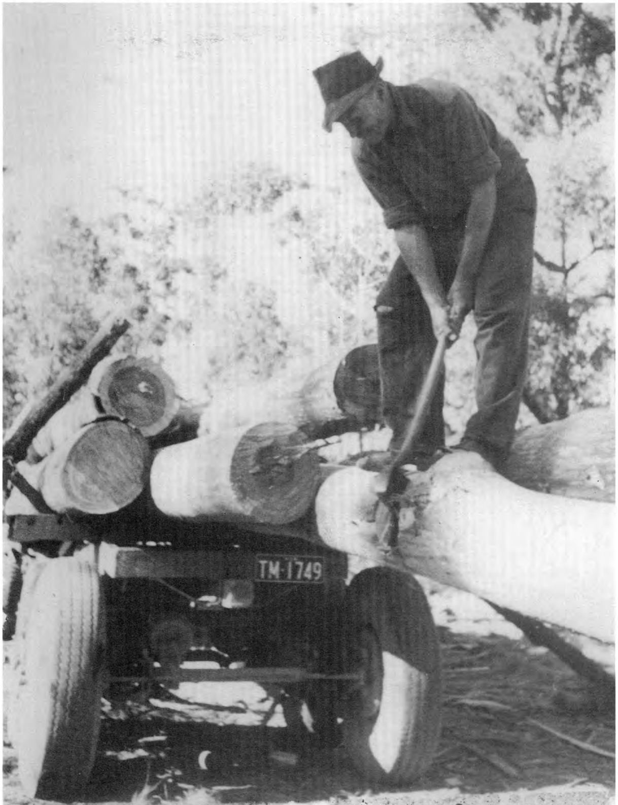
Log being shortened by skilled axeman Matt Lancaster. Matt worked for a time at Newcastle BHP Steelworks cutting piles for foundations for the installation of large machinery. The area being swampland used thousands of piles placed under water level to prevent rot. Concrete was poured on top of the piles. Photo Bert Lancaster.
